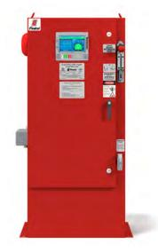
**Description**—Firetrol® FTA1800 Autotransformer Starting Fire Pump Controllers use an autotransformer to supply reduced voltage when starting the motor. The controller is of the closed circuit type where the motor circuit remains closed during the transition from start to run resulting in minimum line disturbance.
